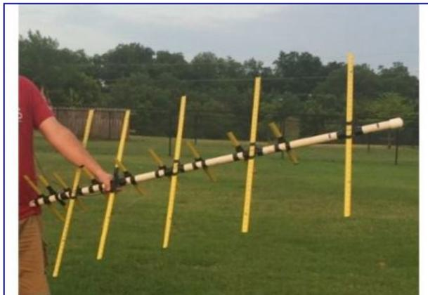
The element holders are attached to the boom with electrical tape in the photo above. While I haven't tried it, I'd suggest that the antenna might be a bit more robust if you could screw or perhaps glue the holders to the boom.
